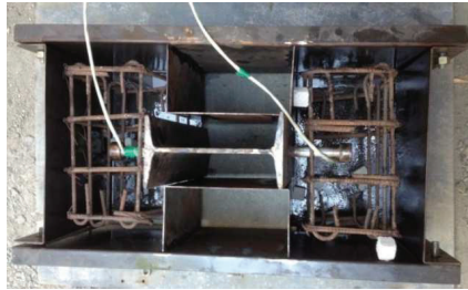
Fig 3. View of concrete casting mould with reinforcements
