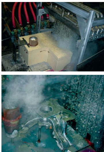
Fig. 2. View of the ablation casting process proposed by Alotech [6]
