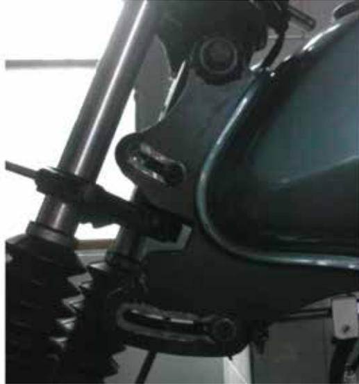
Fig. 5. System changing the angle of steering axis
