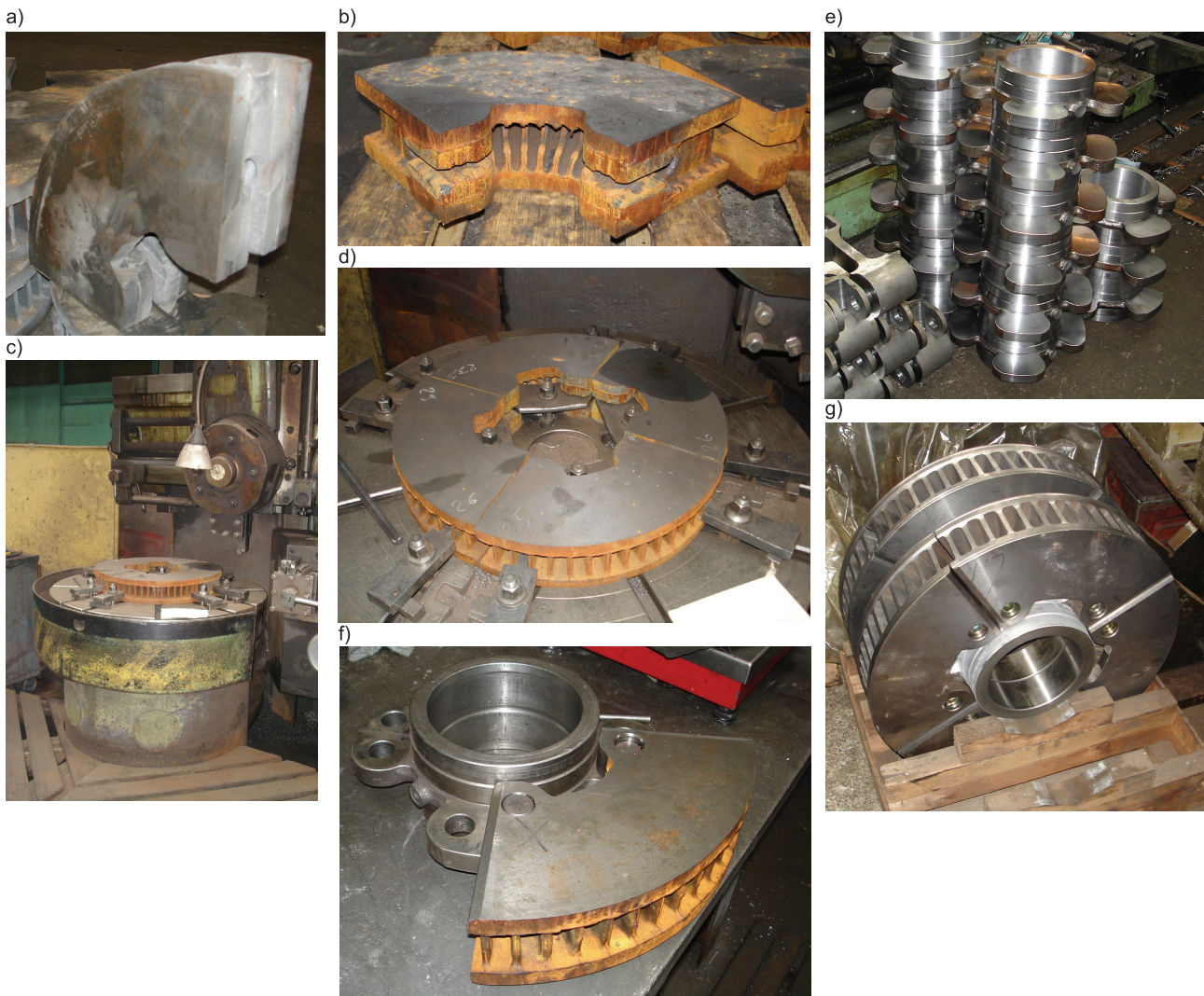
Fig. 4. View of selected stages from the production of segmented brake disc BK 141 mounted on the axle of the wheelset: a), b) view of castings of disc segments divided before machining, c) fixed disc segments on a lathe, d) view of segments on the table of a lathe with pre-machined friction surface, e) view of the brake hub with machined surfaces before drilling assembly holes with segments, f) assembly of segments to the brake hub by means of pins, g) view of the assembled two brake discs [photo. W. Sawczuk]
