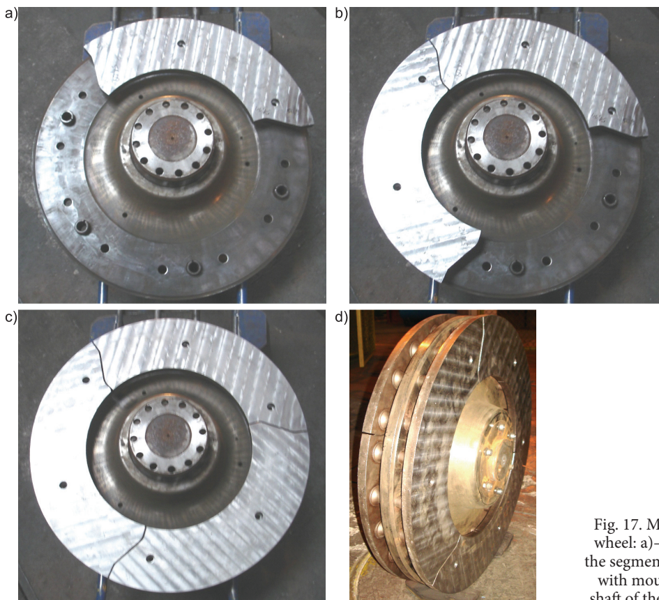
Fig. 16. Steps of making a segmented brake disc: a) connecting disc with rods by welding, b) view after milling the friction surface to size, c) milling the surface of the fan bars [photo. W. Sawczuk]
