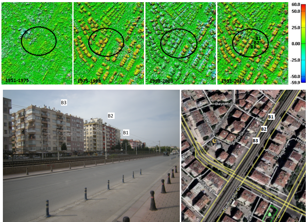
Figure 10. The visualization of changes in comparison of time series point clouds (B1 location: 37^{\circ}53'09.15''N latitude, 32^{\circ}29'08.37''E longitude) (Legend unit: meter)
