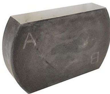
Fig. 1. The sample of 100Cr6 steel after quenching
