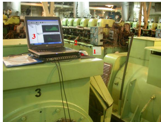
Fig. 1. View of investigated engines and measuring line elements: 1 – test engine, 2 – pressure sensor, 3 – computer
