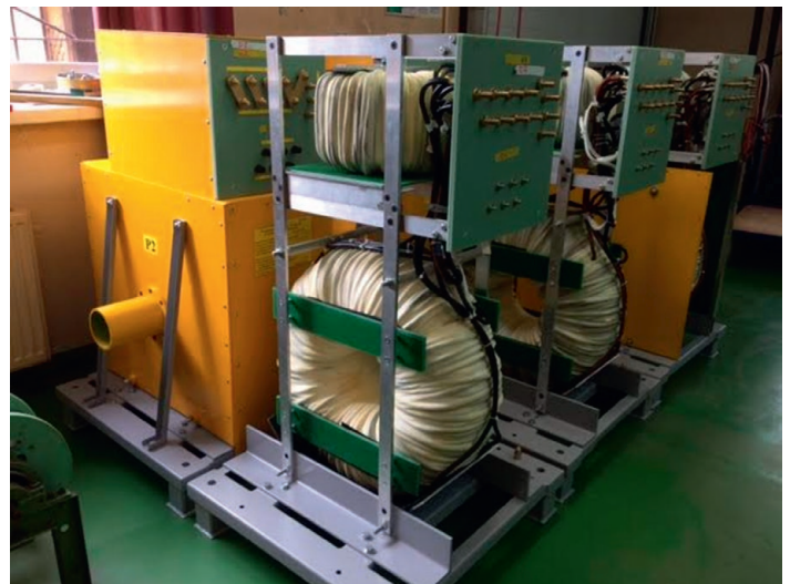
Photo 1. PPZw-30 current transformers, general view
