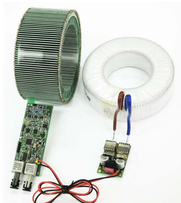
Fig. 2. ISP transducer with autonomous power supply
