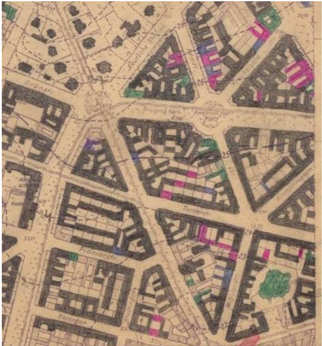
Fig. 2. Inventory of damage in the downtown district of Szczecin – area of the nowadays Szarych Szeregów square and Jagiellońska street. Source: [5]
