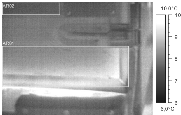
Fig. 3. Thermogram of service heat bridge occurred in the effect of damage in open door leaf when approaching the loading dock
