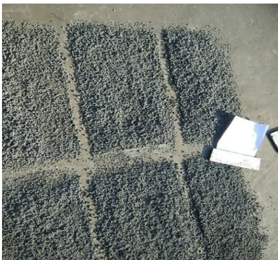
Fig. 4 Product mix found suitable for hydraulic stowing operation
