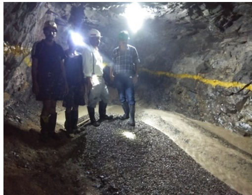
Fig. 7 Compact filling of OB material after 2 hrs at Munsar Mine
