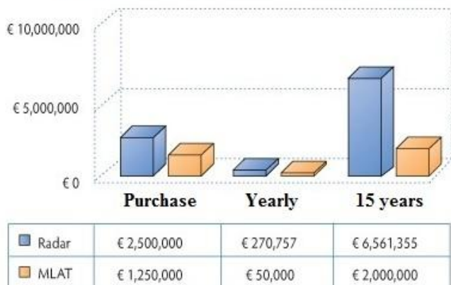
Pict. 1. The comparison of whole operation costs, in case of using of primary radar (PSR), in comparison with MLAT system (PSS).
