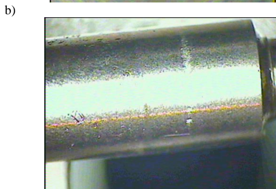
Fig. 5. Cavitation defect in injector overflow valve (a), cavitation defect in pointed follower (b) [8]
