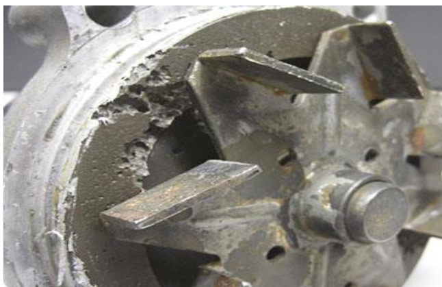
Fig. 2. Cavitation defects with intense characteristic son fixed components of water pump [1]
