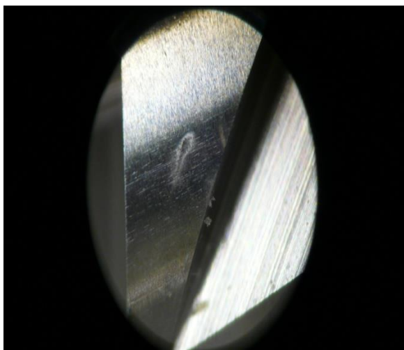
Fig. 4. Plungers in pumping sections (from Bosch) with cavitation pits [8]
