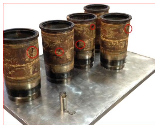
Fig. 1. Cylinder sleeves with cavitation defects - sharp edges of cavitation pits [1]
