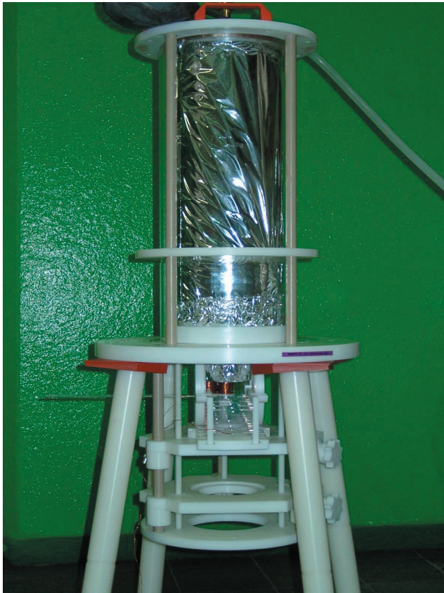
Fig. 2 Two channel SQUID system with polarization and detection coil systems.
