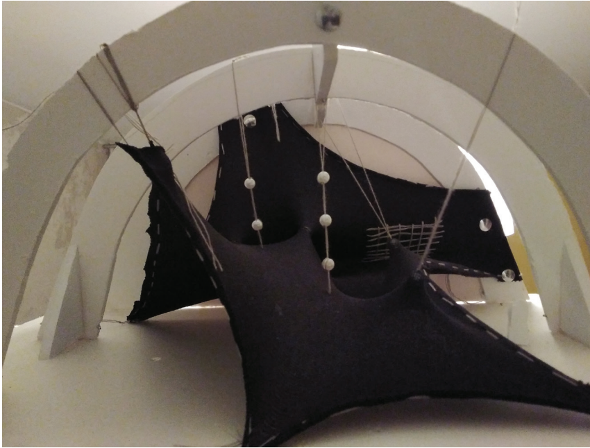
Fig. 6. The form of a membrane platform, stretched to the arches - vertical surface type. This type of platform is much more rigid than the horizontal form and will allow, if implemented, to practice more or less complex climbing. Author: W. Dudek
