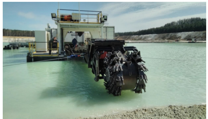
Fig. 1. Suction dredge barge
