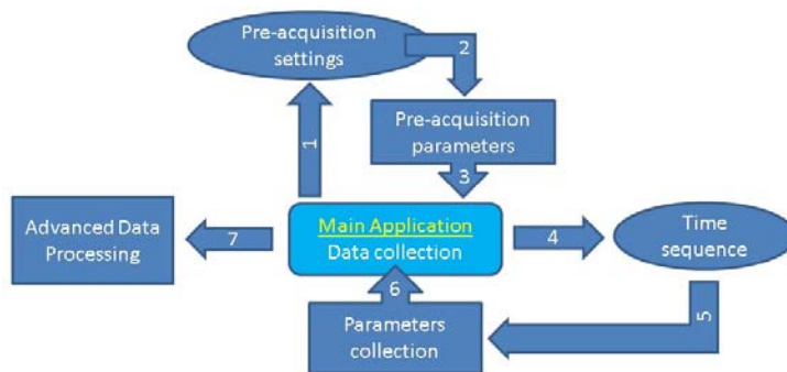
Fig. 8. Simplified block diagram of the TSFF system communication.
