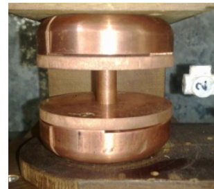
Fig. 4. Setup of the contact system without slits in the contact plates for the flux density measurement (the slits of the two coil parts aligned facing each other)
