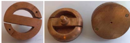
Fig. 3. Unipolar \frac{1}{2} turn contact system, the coil part and the complete contact; the contact plates without slits
