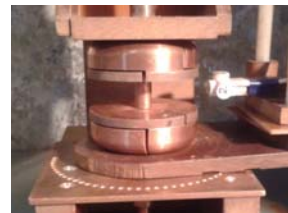
Fig. 8. Setup of the contact system with slits in the contact plates (the slits of the two coil parts aligned facing each other)
