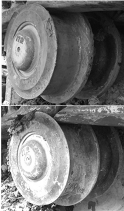
Fig. 4. Upper rollers of bulldozer TD-25M on the open pits Drmno, Tamnava Zapad and Veliki Crljeni after 1205, 1880 and 2242 hours in operation respectively
