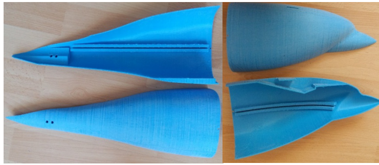
Fig. 1. Model parts printed by FDM
