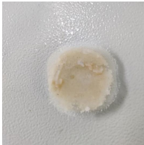
Fig. 5 The phenomenon of "cake forming" in filter screen
