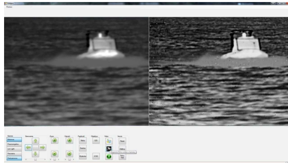
Fig.8. Results of procedure of enhancing imaging processing used in infrared camera: unprocessed image (left), histogram equalization (right).
