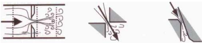
Fig. 16. Different types of holes: orifice and short clearances [32].
