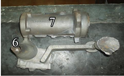
Fig. 8. Casting with redesigned gating and risering systems
