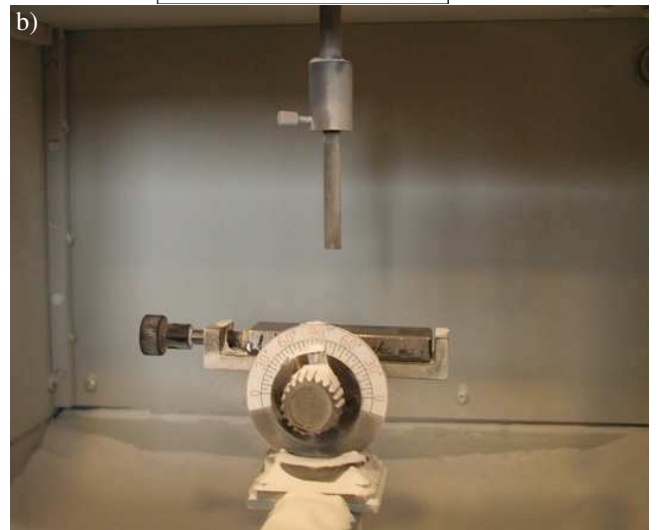
Fig. 3. Erosion resistance test rig according to ASTM G 76-2: a) a schematic view, b) the interior view of the erosion measuring chamber
