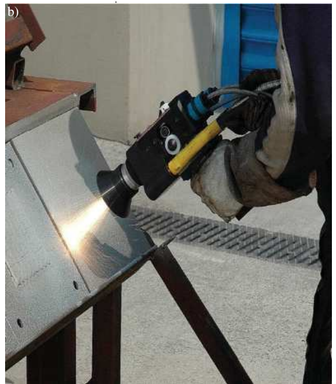
Fig. 2. Arc spraying process: a) a scheme of wire arc spraying apparatus: 1 – compressed air; 2 – wire electric contact; 3 – sprayed layer; 4 – base metal; 5 – electric arc; 6 – wire feeder; 7 – compressed air; 8 – welding wire; b) a photo from trials of arc spraying aluminum coatings with EuTronic Arc Spray 4 equipped with a Gun 4 spray gun
