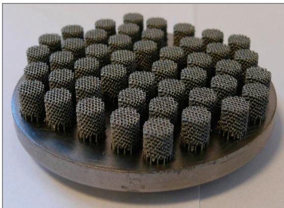
Fig. 1. Scaffolds produced by Selective Laser Melting
