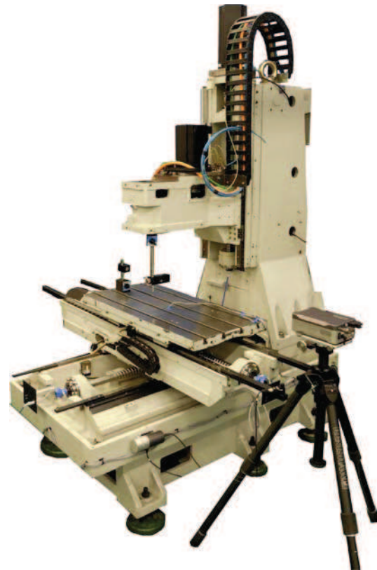
Fig. 4. AVIA VC760 machine tool equipped with screws with temperature sensors during the measurement of positioning accuracy
