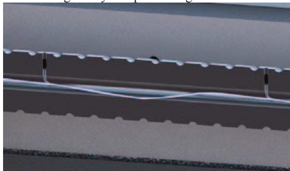
Fig. 1. Visualisation of the NTC sensors mounted in the feed screw
