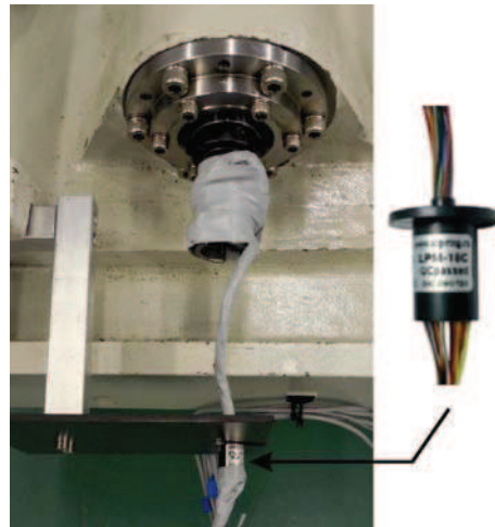
Fig. 2. Photo of the AVIA VC760 machine tool bearing node along with a connector providing the possibility of the sensor system rotation
