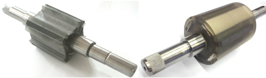
Fig. 1. Initial rotor geometry (without iron poles) consecutive design stages
