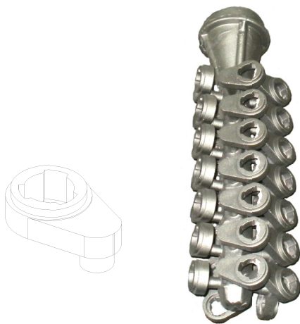
Fig. 4. Carbon steel casts (approximately 0.5% C) in the industrial set after removing FC (next casting sketch)
