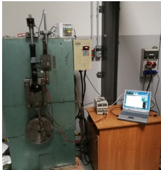
Fig. 5. Bypass-controlled shock absorber mounted on the test stand
