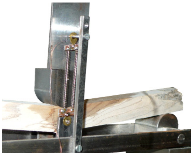
Fig. 11. A stand for measuring wood strength (normal conditions)
