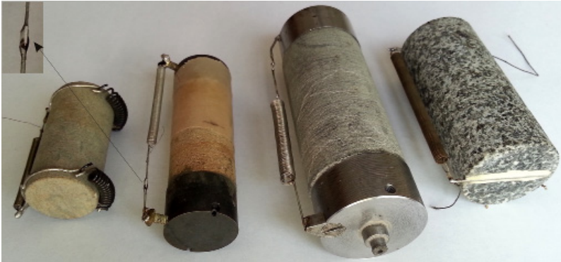
Fig. 6. Various ways of fixing the sensor to rock samples; in the corner, the magnified isolator is visible
