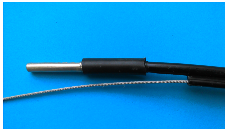
Figure 14. Final/ending sensor on a sensing cable with a security sealing cap. A steel wire is visible, which is later fastened to a leading cone during cable ground installation.
