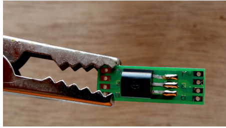
Figure 13. Intermediate sensors mounted along the cable with a dedicated PCB (printed circuit board).
