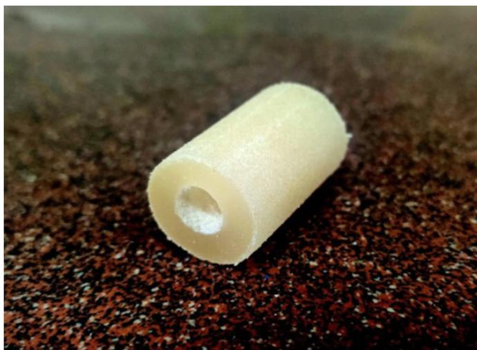
**Figure 8.** The shape of a sample for testing the propellant burning rate
