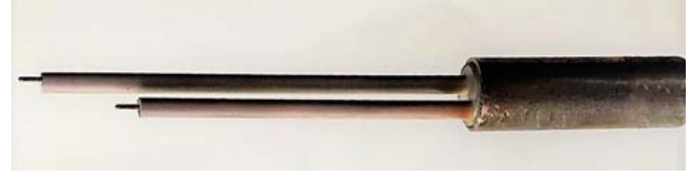
Fig. 5. The probe used for the measurements of the electric field radial component.
