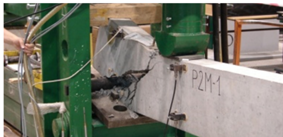
Fig 6. Failure of a reinforced concrete beam with insufficient bond length in the support zone of the main tensile reinforcement [18]
