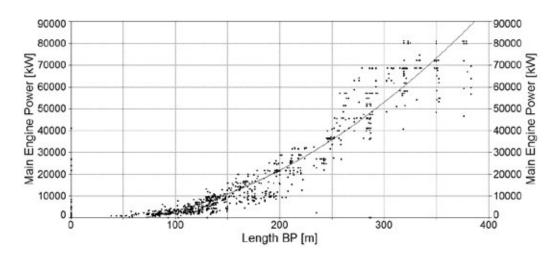
Fig. 2 Approximations of main engine power on length between perpendiculars, relationship (3) in comparison with reference data
