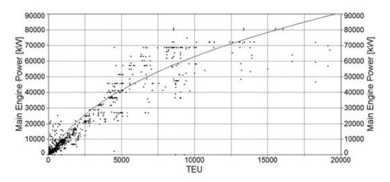
Fig. 1 Approximations of main engine power depending on the number of containers, the relationship (2) in comparison with reference data
