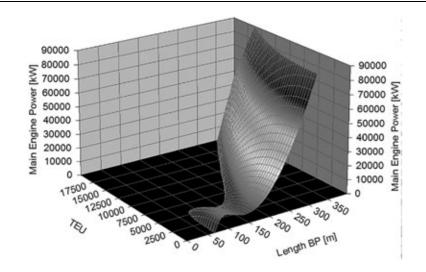
Fig. 3 Projecting the main engine power of a container ship depending on the length between perpendiculars and TEU capacity according to formula (4)
