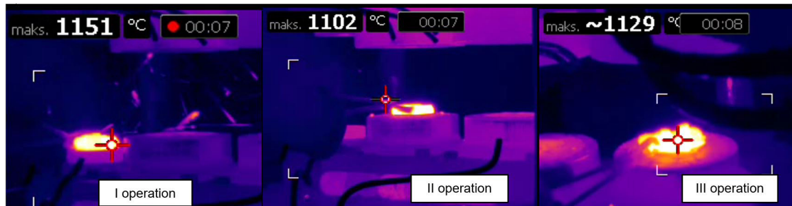
Fig. 5. Temperature measurements made after the consecutive operations of flattening, preliminary and finishing forging
