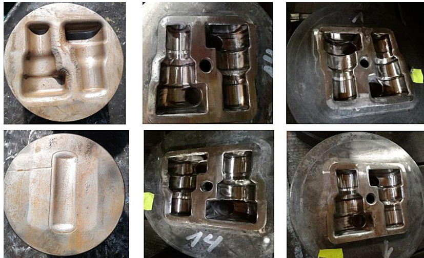
Fig. 4. Image of the particular die inserts used in the process of producing an adapter forging
