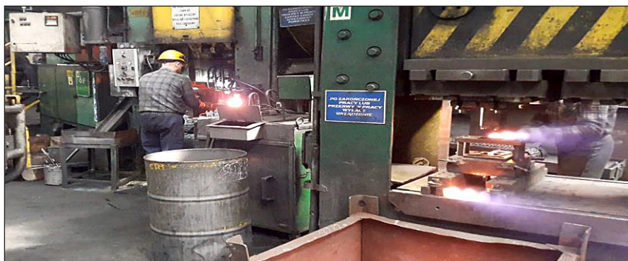
Fig. 3. View of the technological line: left – the die forging process on a press Masey, pressure 13MN, right – the process of hot trimming of the flash on a trimming press
