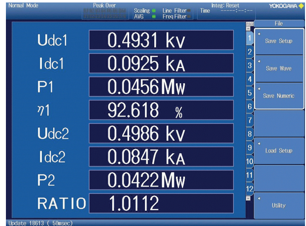
Fig. 14. Stationary parameters measured by Yokogawa on the test stand for transferred power P = 45,6 kW and efficiency 92.6%
