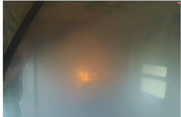
Fig. 6. Passenger coach after approx. 3 minutes of water mist spraying. The visibility is strongly reduced [5, 16]
