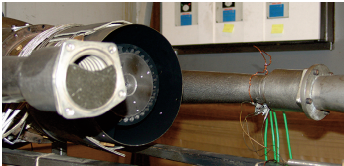
Fig. 16. Picture of modified chamber of engine GTD-350 [Gut, 2013].
