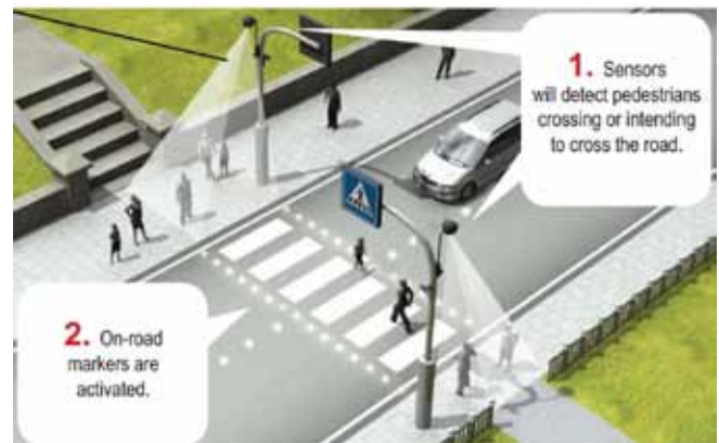
Fig.5. System SAFE-2-WALK by Traficon
