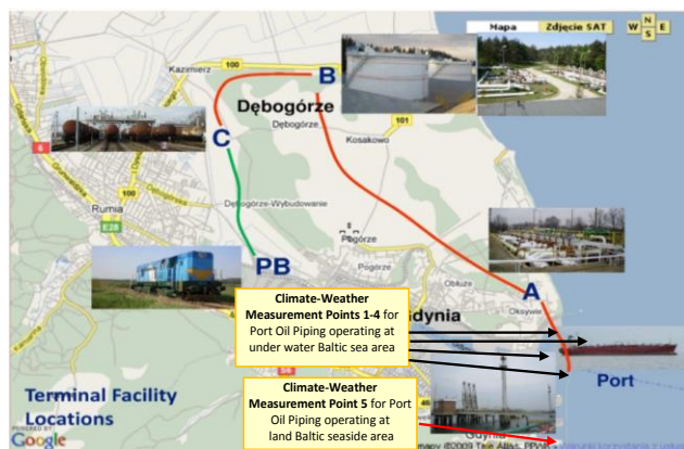
Figure 2. The port oil piping transportation system operating between the Port of Gdynia and the Terminal in Dębogórze
