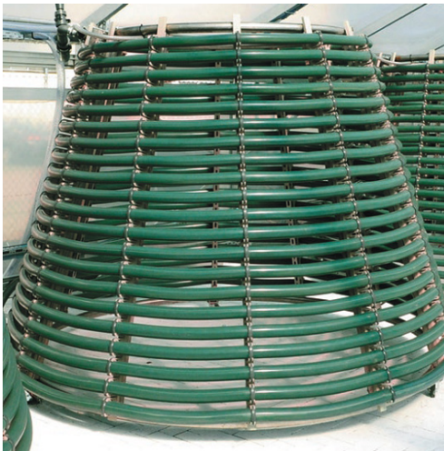
Fig. 2. Truncated cone shaped light collector (“Christmas tree” GICON-PBR) (Posten et al., 2018)
