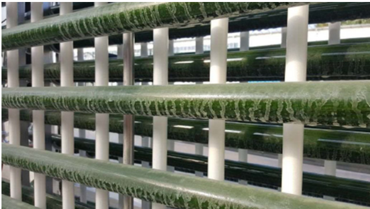
Fig. 4. Scaling of light entry surface of glass tubular PBR (photo: S. Matthes)
