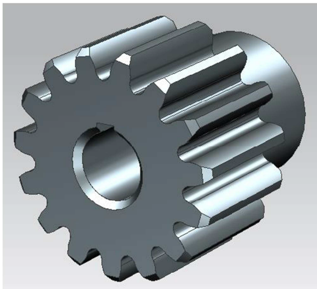
Fig.2. The example of the 3D model of gear: m = 2 , z = 15 , y = 1
