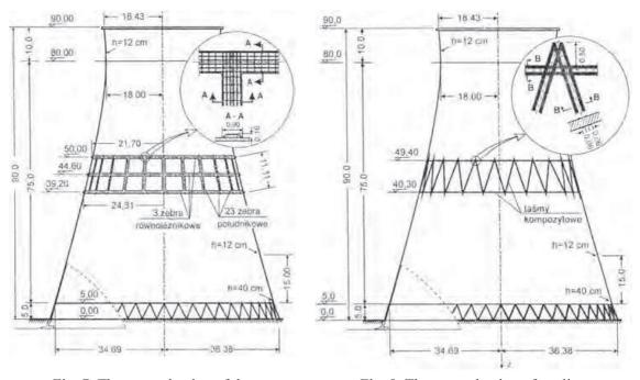
Fig. 7. The strengthening of the cooling tower shell by reinforced concrete ribs - the first variant [9]
