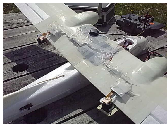
Fig. 8. Test UAV with two laser rangefinders fixed to its wings
