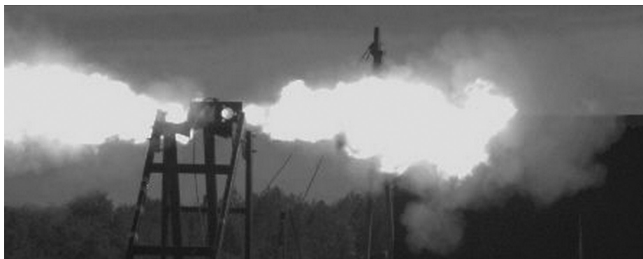
Figure 2. Propellant gases flowing from the barrel through the holes during firing
