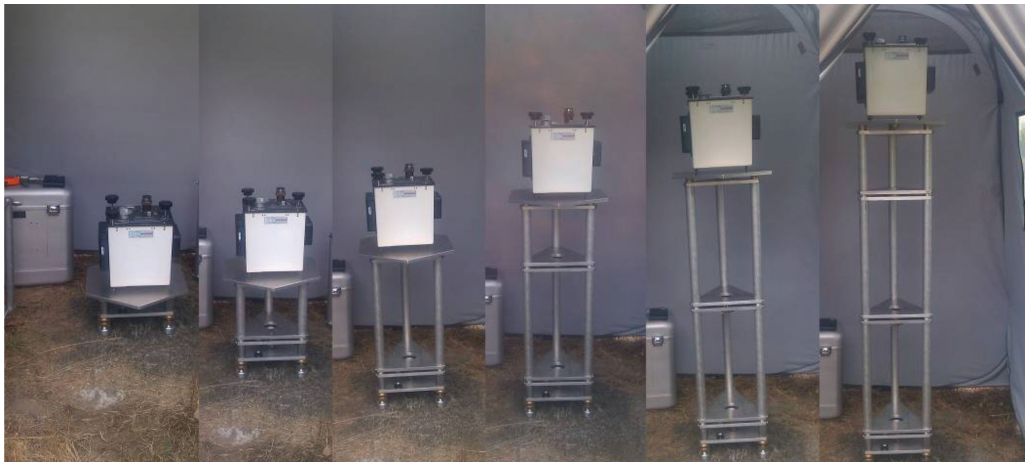
Fig. 6. Gravity measurements at a field station for vertical gravity gradient determination with the use of the stand constructed in the Institute of Geodesy and Cartography, Warsaw
