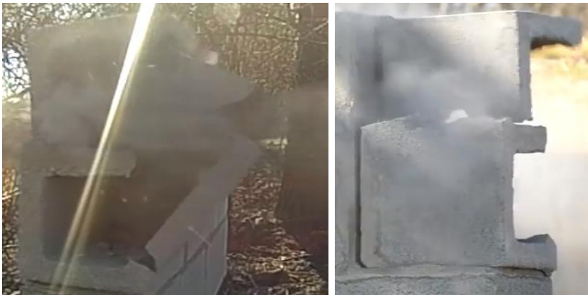
Fig. 10. The effect of a real Special Forces Short Magnum strike, front and lateral view
