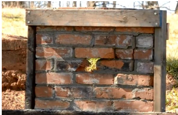
Fig. 6. A real brick wall after being hit by a projectile
